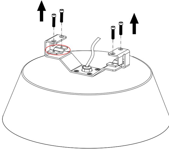
**2** Hang the fixture into the steel wire
